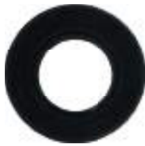
RETENTOR BORRACHA 30,0 X 55,0 X 8,0MM cód. 3110310007 | unid. PC
